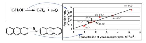
An excellent correlation between the activity of anion-doped alumina catalysts in ethanol dehydration and the concentration of weak acceptor sites capable of ionizing anthracene has been observed.
