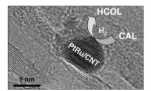
Very active and selective Pt-Ru/CNT catalysts have been prepared for the selective hydrogenation of cinnamaldehyde into cinnamyl alcohol. Characterization using HRTEM, WAXS and EXAFS was indicative of the influence of particles alloying on the selectivity of these systems..
