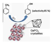
Mesoporous gallium phosphates synthesized by hydrolysis of gallium alcoxide in the presence of PCl<sub>3</sub> assisted by surfactants form robust structures exhibiting the potential of the aerobic oxidation of toluene.
