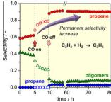
Temporary addition of CO during propyne hydrogenation on a copper catalyst permanently boosts the propene selectivity by inducing a smaller ensemble that cuts down the oligomerization path.
