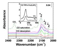
Unexpectedly, CO interacts rapidly with Au/LaPO<sub>4</sub> to evolve CO<sub>2</sub> even though the LaPO<sub>4</sub> is non-reducible. H<sub>2</sub> evolves with CO<sub>2</sub> during CO-TPR of Au/LaPO<sub>4</sub> (but not for Au/FePO<sub>4</sub>) so surface hydroxyls react to oxidize CO, catalyzed by the Au, a pathway competing with direct CO oxidation.
