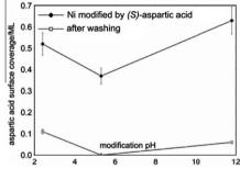
Ni catalysts modified by (S)-aspartic acid exhibit a sharp maximum in enantioselectivity following modification at pH 5.0 and 300 K. XPS shows that under these conditions the coverage of aspartate is vanishingly small implying that enantioselectivity, in this case, may be derived from chiral metal sites created by the corrosive leaching of Ni by aspartic acid.
